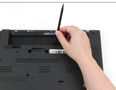
• Use the spudger to pry up the bottom cover in the lower portion of the external battery compartment by a few millimeters.
