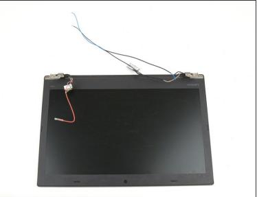
Use both of your hands to lift the bottom of the laptop away from the LCD assembly.
