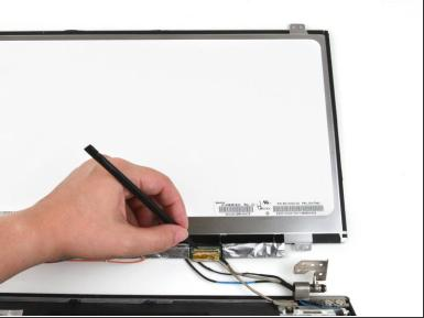
Use the pointed end of a spudger to flip up the metal bar securing the connector.
