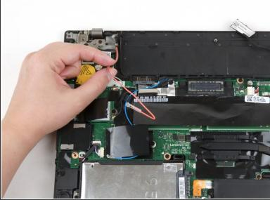
• Use your fingers to remove the gray and red coaxial cables from their slots along the motherboard.
