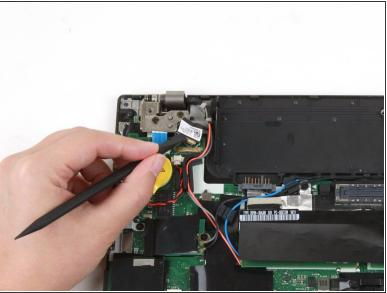
• Use the flat end of a spudger to detach the camera/microphone cable connector from its socket.
