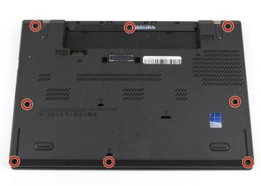
Loosen the eight captive screws in the bottom cover using a Phillips #1 screwdriver.
