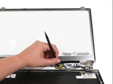
Use the flat end of a spudger to disconnect the display cable from its socket.
