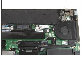
Use a pair of tweezers to lift the LCD cable bracket away from the motherboard.
