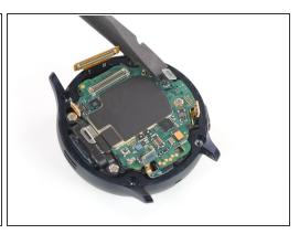
Use a spudger to disconnect the barometric sensor, the buttons, and the microphone.
