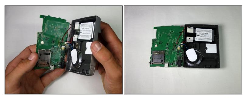
• The motherboard will now freely separate from the back casing; lay it flat next to the housing.
