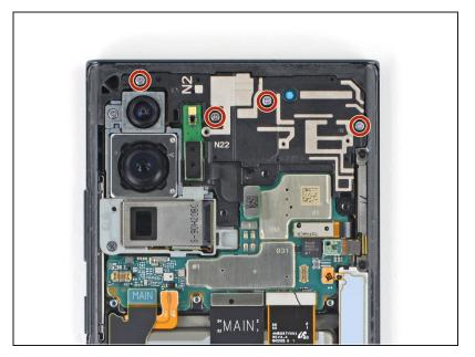
Use a Phillips screwdriver to remove the four 4.0 mm screws securing the earpiece speaker.
