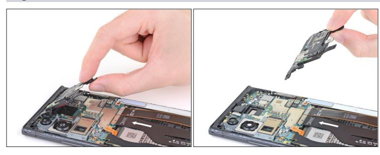
• Lift and remove the earpiece speaker.
