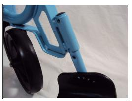
Slide the footrest sockets down as shown and use a 10 mm wrench to tighten the bolts at the desired height.
