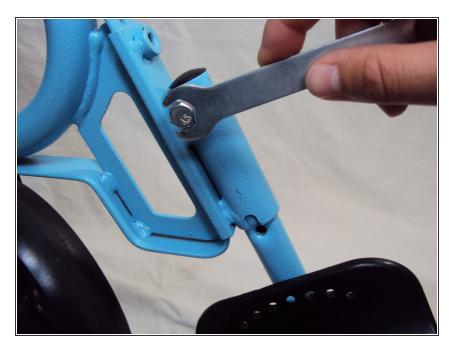
Screw in the bolt to the top socket to secure the height of the footrest.
