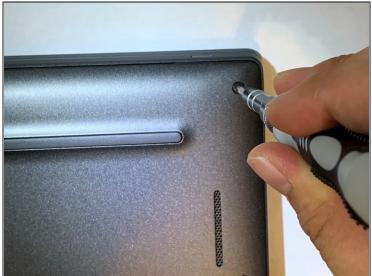
• Remove the eight 7 mm screws from the from the back panel using the Phillips #1 screwdriver.
