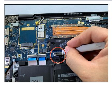
Disconnect the battery from the motherboard by gently pulling out the connector.
