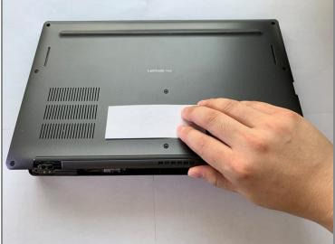
Slide the opening pick in between the back cover and work your way around the edges to remove the back cover from the device.
