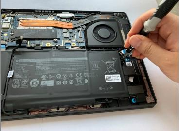
Using the Phillips #1 screwdriver, remove the five 5 mm screws.
