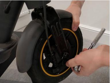
To detach the brake, use a 10 mm Allen wrench to remove the bolt from the tire that is attached with the brake.
