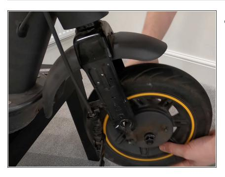
Pull down the tire and remove it from the frame.
