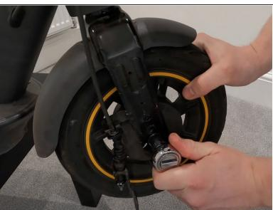
Use a 15 mm socket wrench to remove 15mm bolt from the tire of the scooter on both sides of the front wheel.
