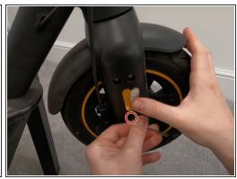
Use 3 mm Allen key to loosen three hexagon screws from each side of the wheel.
