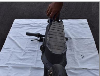
Flip the scooter upside down and unscrew the 18 screws holding the base plate using a Security Torx T15 screwdriver.
