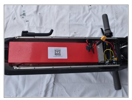
Place the new battery inside the enclosure and reinstall the 10 screws (if needed), bonding the battery to the scooter.
