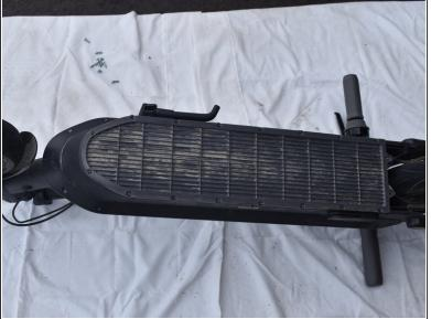
• Line up the base plate and tighten it with all 18 screws using a Security Torx T15 Allen Key.
