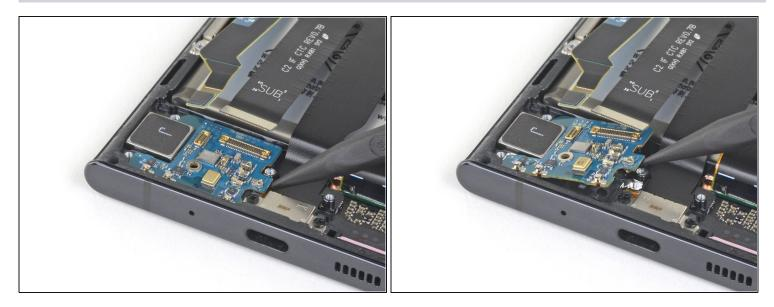
(i) The daughterboard is fitted to the frame by three spring connectors along its bottom edge.
