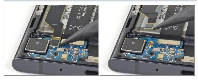
• Use the pointed end of a spudger to disconnect the secondary interconnect cable from the daughterboard.
