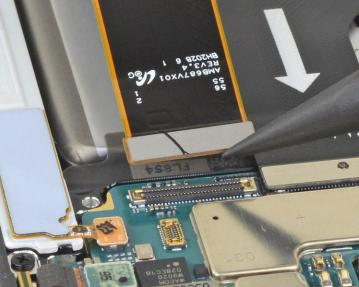
Use the pointed end of a spudger to disconnect the display cable from the motherboard.
