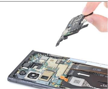
• Lift and remove the earpiece speaker.
