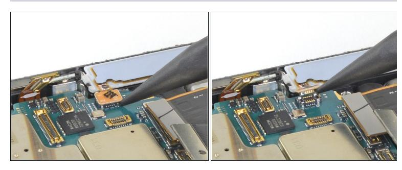
• Use the pointed end of a spudger to disconnect the S-Pen press connector from the motherboard.
