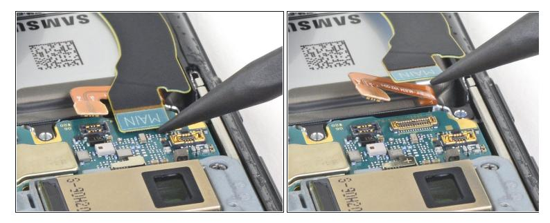
• Use the pointed end of a spudger to disconnect the secondary interconnect cable from the motherboard.
