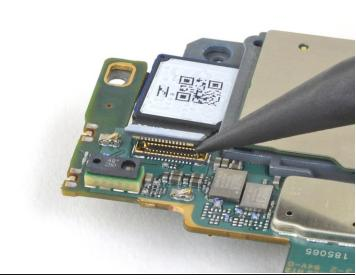
• Use the pointed end of a spudger to disconnect the ultra wide camera from the motherboard.
