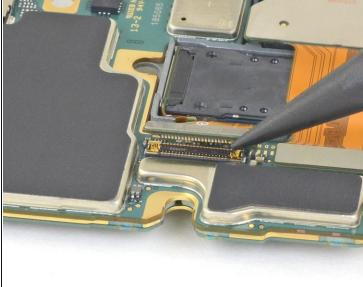
• Use the pointed end of a spudger to disconnect the telephoto camera from the motherboard.
