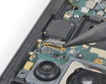
• Use the pointed end of a spudger to disconnect the front-facing camera cable from the motherboard.
