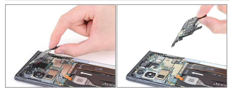
• Lift and remove the earpiece speaker.
