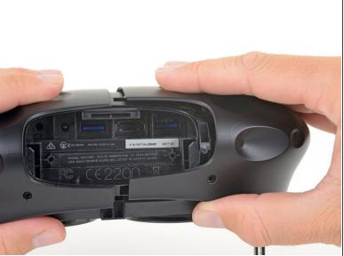
Grasp the right half the outer shell and pull it to the right and toward the front of the headset in a twisting motion until you feel the clips on the front of the cover release.
