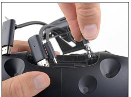
Repeat the lifting and unplugging process with the remaining USB, power, and audio cables.
