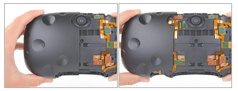
Repeat the last three steps for the left side of the outer shell and remove it.
