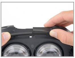
Grasp the top edge of the right half of the outer shell, behind the component cover and near the seam in the center. Pull it to the right and upward, away from the headset to release the clip securing that part of the shell.
