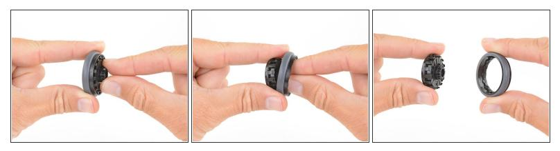
Push the internal locking mechanism out of the grip.
