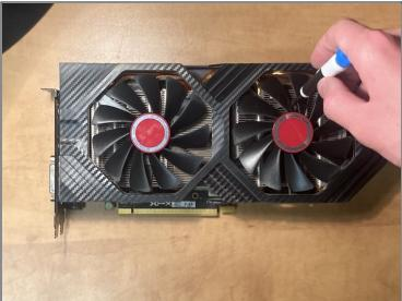
• Remove the six 1.8 mm screws holding both fans in place by using a Phillips #1 screwdriver in-between the fan blades as the screws are located behind the fans.
