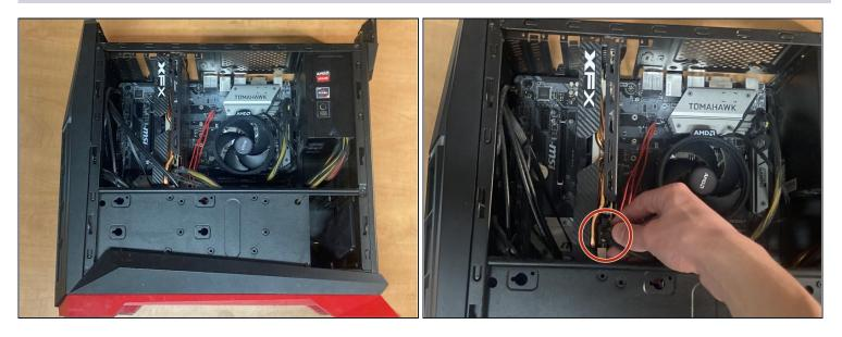
To disconnect the GPU cable, use your thumb and index finger to unlatch the hooking device and pull the cable away.
