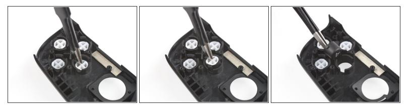
• Use a pair of tweezers to remove the face buttons.
