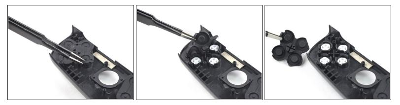
Use a pair of blunt nose tweezers to remove the rubber cover which is placed over the face buttons.
