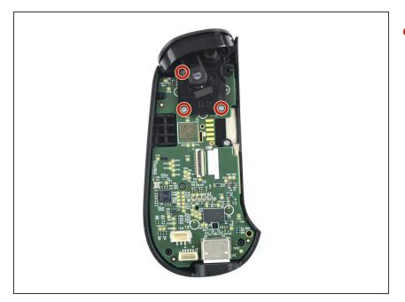
• Use a Phillips screwdriver to remove the three 5.9 mm-long screws.
