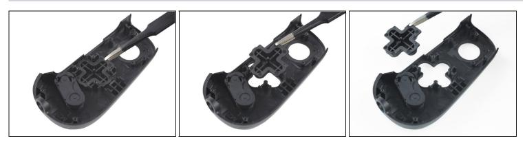
• Use a pair of blunt nose <u>tweezers</u> to remove the direction pad.
