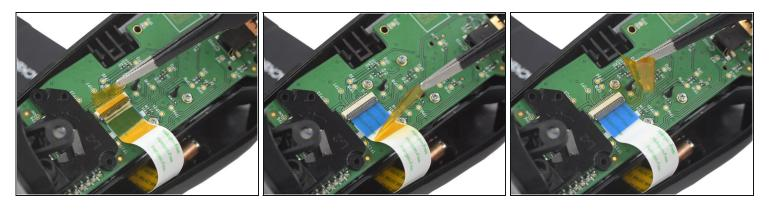
• Use a pair of <u>tweezers</u> to remove the yellow protective tape which is placed over the interconnect cable connector.
