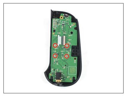
Use a Phillips screwdriver to remove the four 3.9 mm-long screws.
