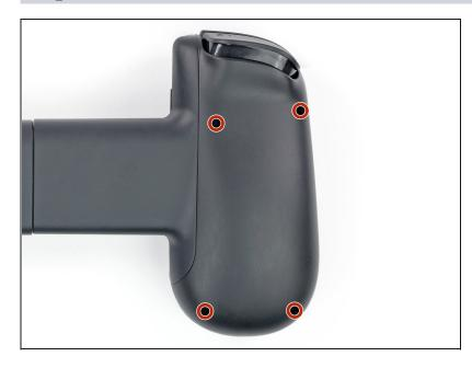
Use a Phillips screwdriver to remove the four 5.9 mm-long screws.
