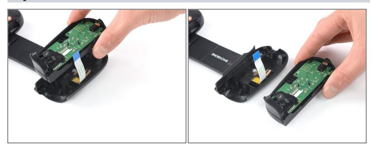
• Remove the upper half of the left controller assembly.
