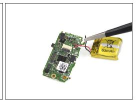
Use a soldering iron to desolder the first battery cable from the motherboard.
