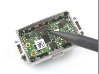
Use the pointed end of a spudger to pry up and disconnect the heart rate monitor sensor flex cable.
