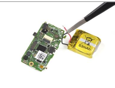
Use a soldering iron to desolder the second battery cable from the motherboard.
