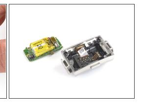
Use an opening pick to pry up and remove the motherboard which is holding the battery.
