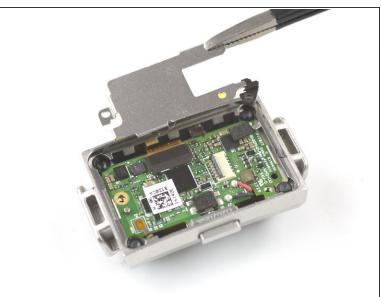
Use a pair of blunt nose tweezers to remove the motherboard shield.
