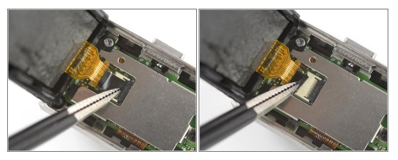
Use a pair of blunt nosed tweezers to remove the black sticker which covering the touch screen connector.
