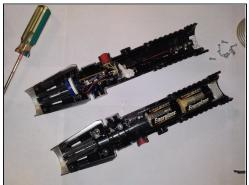
• Use a Phillips #2 screwdriver to remove the 3.5 mm screws on the hilt.
