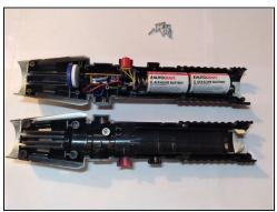
• Place the new C batteries inside the newly cleaned hilt.
