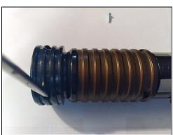
• Use your Philips #2 screwdriver to screw the 3.5 mm screws back into the hilt.
