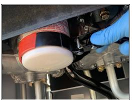
Using a filter wrench, twist counter-clockwise to remove the old filter.
