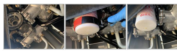
Once the filter has been removed, place the new filter over the housing and screw clock-wise to install.
