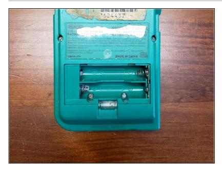
Remove the battery cover and batteries.
