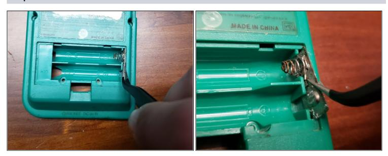
• Using a pair of tweezers, remove the battery terminal from the shell.
