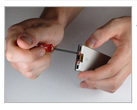
Remove the two screws shown using a Y00 Tri-Wing screwdriver.
