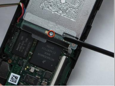
Remove the single screw under the battery using a small Tri-Wing screwdriver.
