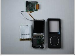
Remove the faceplate by using a metal spudger to separate it from the remaining components.
