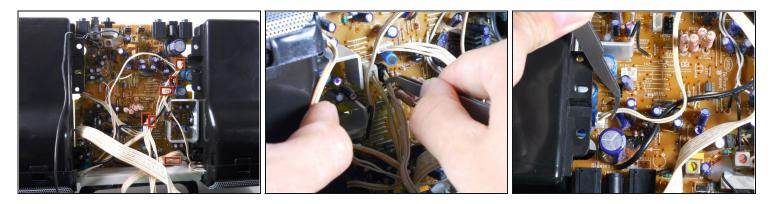
• With the back of the iHome is facing you, tilt the Motherboard Assembly upwards as shown.
