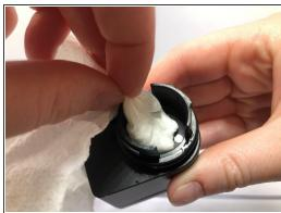
Wipe the shaft and the cavity with a damp paper towel to remove vinegar.
