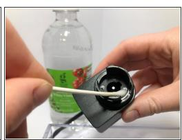
• Clean the shaft and the cavity with Q-tips dipped in vinegar in a scraping motion.
