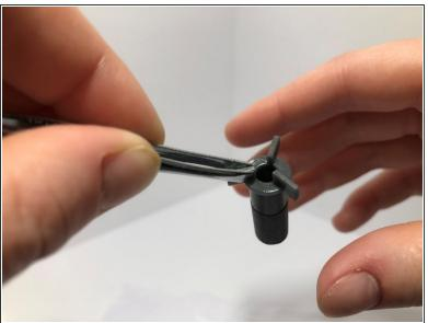
Pick up the new impeller using tweezers.
