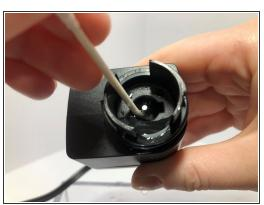
Swirl the cavity with a Q-tip to scrape off any build up of sand or organic material.
