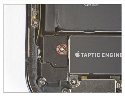
• Use a Phillips driver to remove the 1.4 mm screw securing the Taptic Engine plastic cover.
