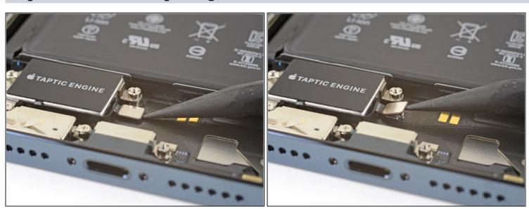
• Use the point of a spudger to pry the Taptic Engine connector straight up and out of its socket.
