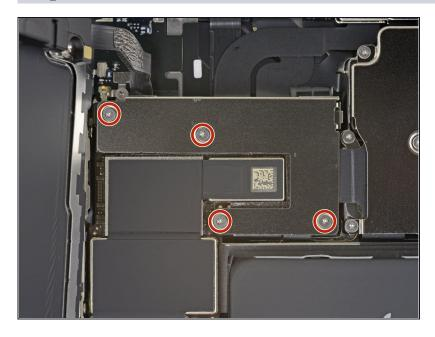
Use a Y000 driver to remove the four 1.1 mm-long screws securing the front sensor connector cover.
