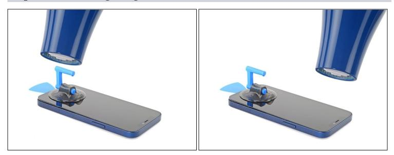
• Use a hair dryer to heat the right edge of the iPhone (the edge with the power button) for 90 seconds or until the screen is slightly too hot to touch.
