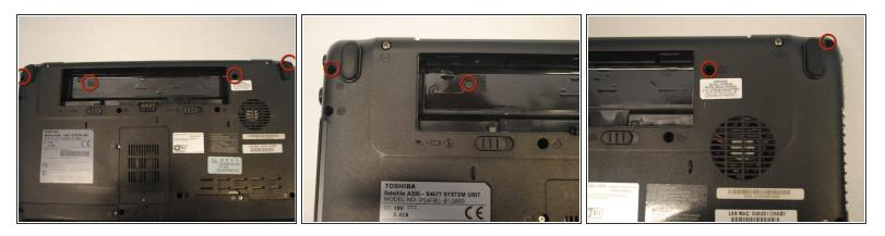
Remove the four screws indicated in the photos using a Phillips 00 Screwdriver. Left to right: 6mm button-head, 3mm flat-head, 6mm button-head, 6mm button-head.
