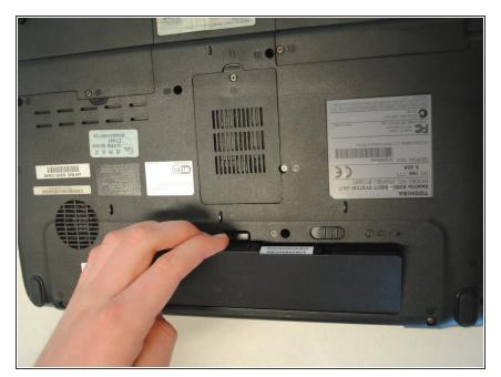
• While holding the left lock, place your finger in the indentation next to the battery and lift the battery out.
