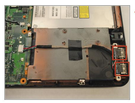
• Locate the USB 2.0 cable on the bottom right corner of the laptop.
