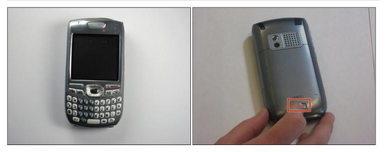
• Remove the battery cover by pressing on the small rectangular button located on the back of the phone.
