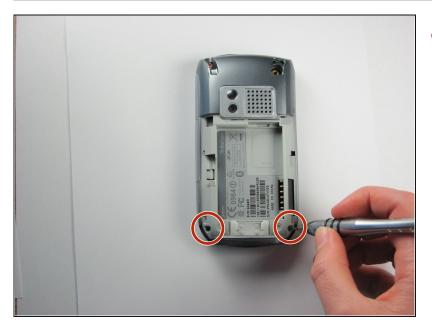
Remove the remaining two 27mm screws from the bottom using the T6 screwdriver.
