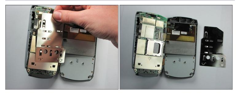
• Slide the slim metal plate upwards until it disconnects from the motherboard.
