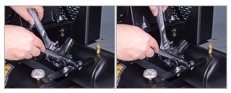
• Push the adjustable wrench to break the regulator loose from the threaded nipple.
