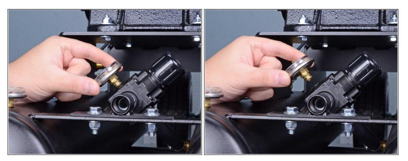
• Remove the pressure gauge.
