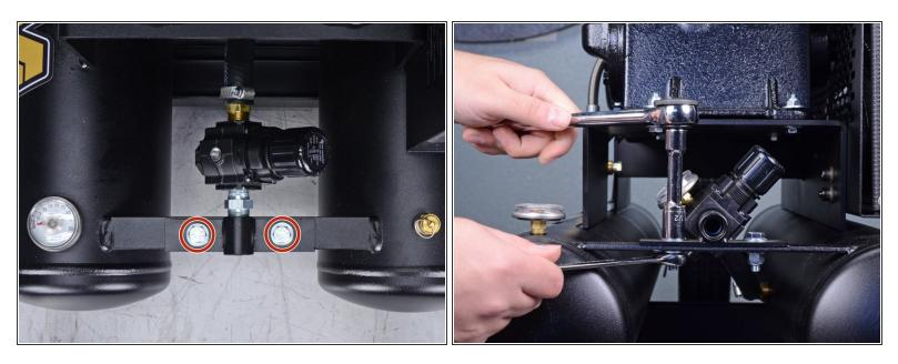
• Use a 1/2 inch socket and wrench to remove the two bolts and accompanying nuts securing the regulator mounting bracket to the frame.
