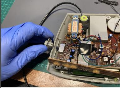
Remove the ALARM ON/OFF button
