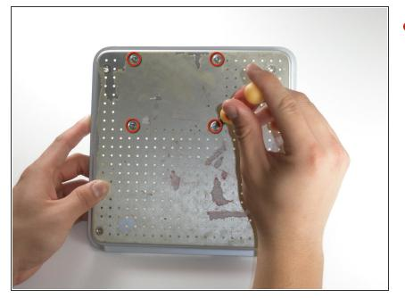
Remove the four T8 Torx screws securing the hard drive to the lower case.
