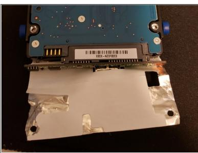
Carefully peel away the shielding
