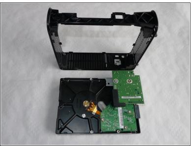
Slide out the hard drive as shown in the picture
