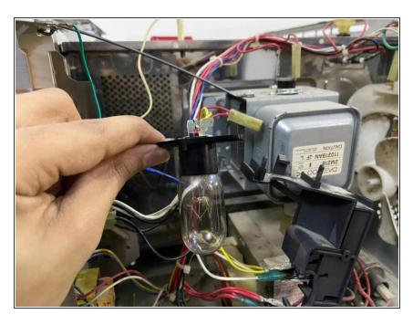
Remove the screws that hold the lightbox in place with a Phillips #0 screwdriver.
