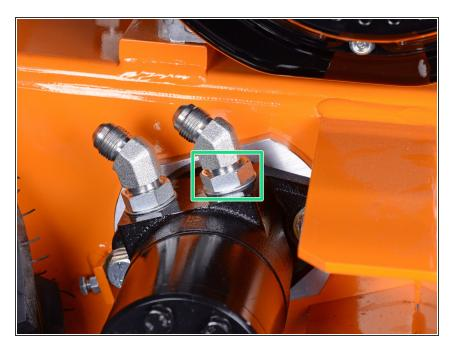
Use an adjustable wrench to loosen the nut locking the upper hose fitting to the wheel motor.
