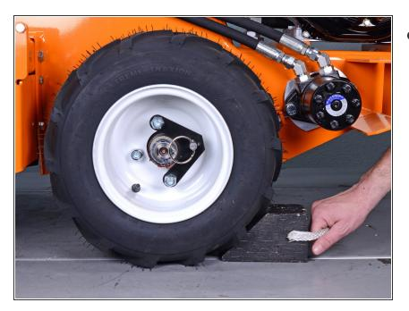
Insert wheel chocks underneath each wheel to keep the device stationary during disassembly.
