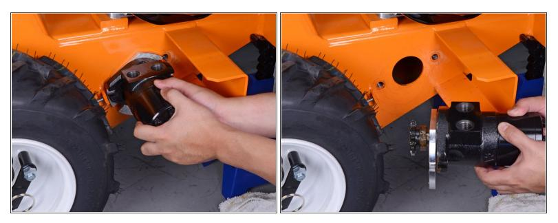
• Remove the wheel drive motor, spacer, and sprocket assembly.
