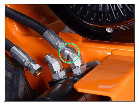
Use an adjustable wrench to loosen the nut securing the upper fluid hose to the fitting on the wheel motor.
