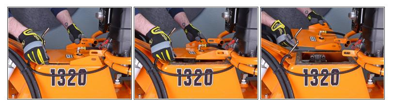
• Lift the tank lid out and around the engine guard mounting tabs to remove it.
