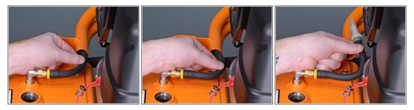
• Remove the end of the tank breather tube from inside the engine guard structural pipe.
