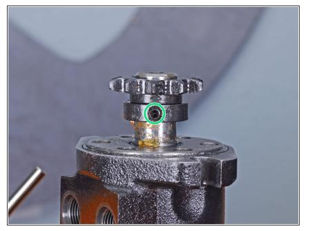
Use a 5/32 inch hex key to loosen the set screw securing the sprocket to the wheel motor shaft.
