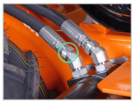
• Use an adjustable wrench to loosen the nut securing the lower fluid hose to the fitting on the wheel motor.
