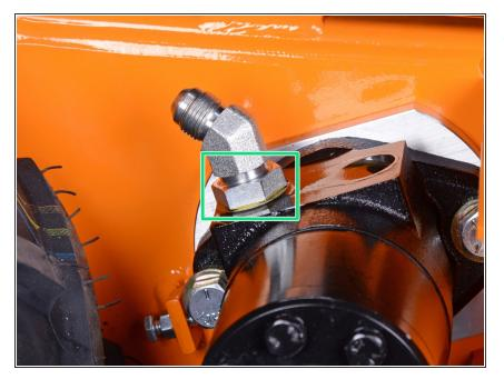
Use an adjustable wrench to loosen the nut locking the lower hose fitting to the wheel motor.
