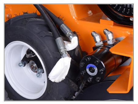
Place paper towels into the hose openings to block residual fluid from dripping as you continue the procedure.
