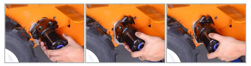
With the motor loose, rotate it 90° counterclockwise and push it as far left as it will go to give the drive chain some slack.
