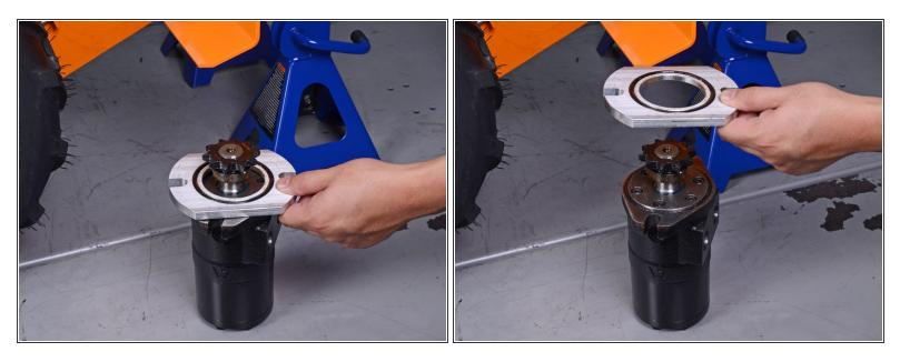
• Remove the wheel motor spacer.
