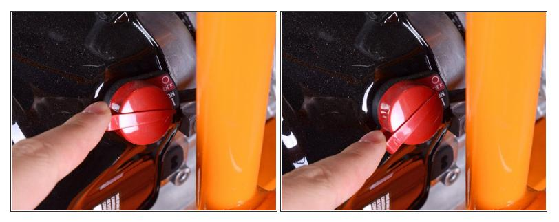
• Flip the red engine ON/OFF switch to the **OFF** position.
