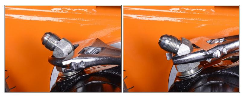
• Use an adjustable wrench on the fitting body to unthread it from the wheel motor.
