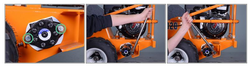
Use a 3/4 inch socket and breaker bar to remove the two bolts securing the wheel drive motor to the frame.
