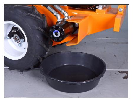
Place an oil drain pan underneath the wheel drive motor to catch hydraulic fluid that will spill out during this procedure.
