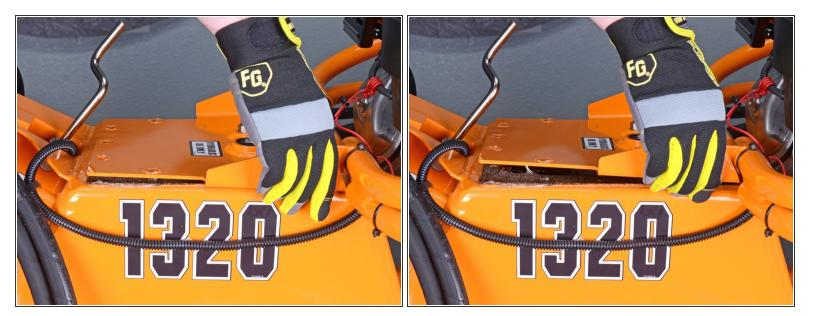
• Lift up on the lid to break the seal around the perimeter of the gasket.
