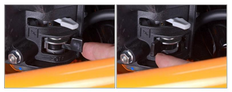
• Flip the fuel valve lever to the **OFF** position.
