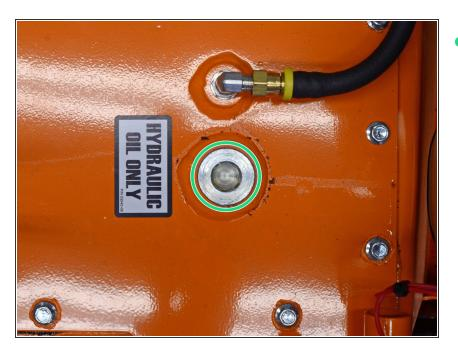
Use a 14 mm hex key to remove the tank fill plug.
