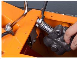
**Reassembly tip:** In order to bring the plunger assembly backwards, up and over the tank edge, use an open-ended wrench to compress the plunger assembly while rotating the actuator valve.
