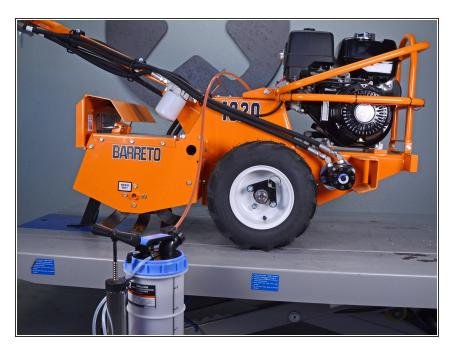
Use a siphon to pump out as much fluid as you're able to, totaling about 14 gallons.
