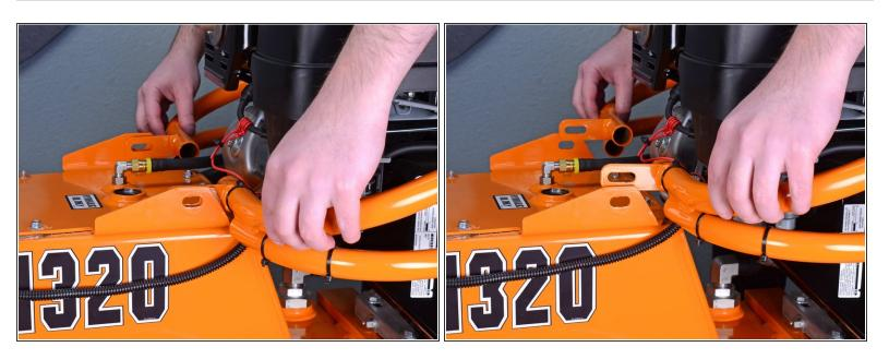
Lift the engine guard up above the tank lid flanges.
