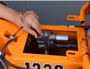
Rotate the actuator valve so the return tube and relief valve are horizontal and parallel to the tank opening, facing the engine.
