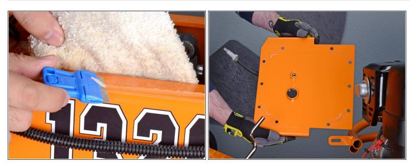
Before reinstallation, remove all remnants of old silicone gasket from both the rim of the fluid tank as well as the tank's lid.
