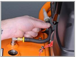
Remove the end of the tank breather tube from inside the engine guard structural pipe.
