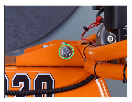
Use a 9/16 inch socket and wrench to remove the two bolts and accompanying nuts securing the engine guard to the tank lid, one on each side.
