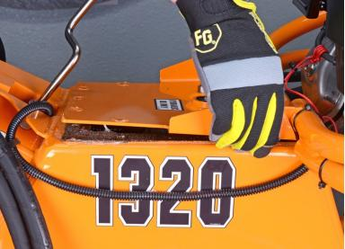
• Lift up on the lid to break the seal around the perimeter of the gasket.
