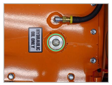
Use a 14 mm hex key to remove the tank fill plug.
