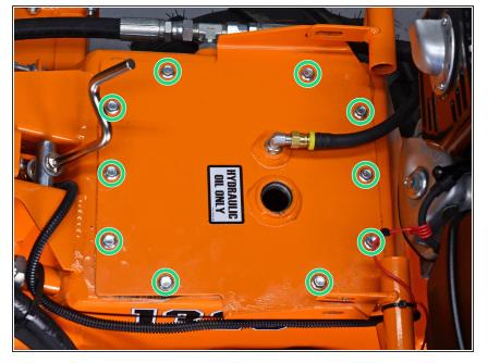
Use a 3/8 inch socket to remove the ten bolts securing the tank lid.
