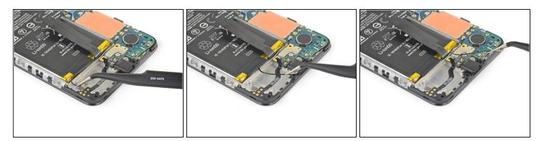
• Use your fingers or a pair of tweezers to pull the antenna cable out from underneath the tape covering it.
