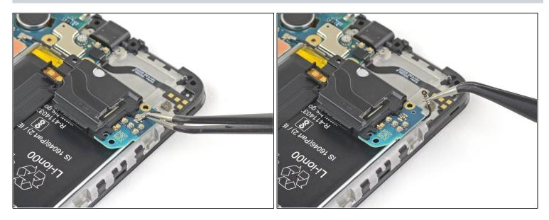
• Use a pair of tweezers to disconnect the antenna cable from the loudspeaker assembly.
