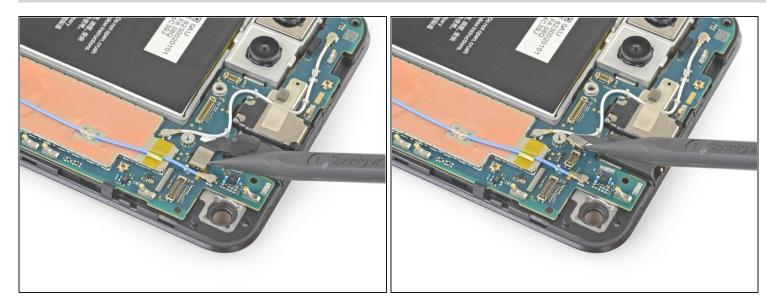
• Use the tip of a spudger to disconnect the headphone jack cable from the motherboard.
