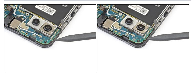
(i) The motherboard is secured to the midframe by plastic clips.
