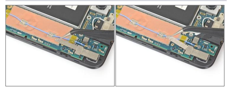
• Use your fingers or a pair of tweezers to peel the tape off of the copper foil.
