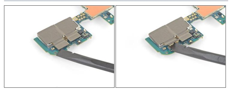
• Use the flat end of a spudger to disconnect the left camera from the motherboard.
