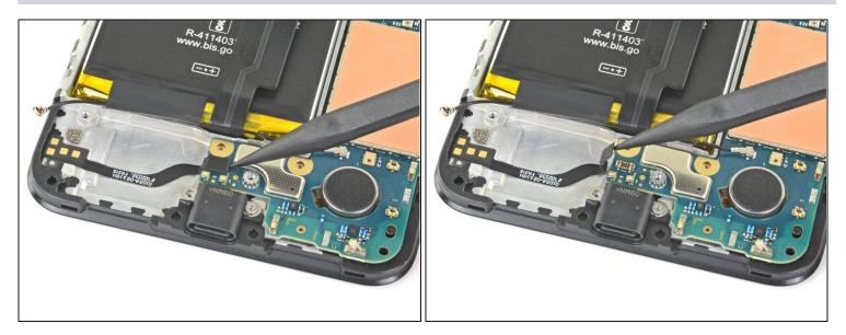
• Use the tip of a spudger to disconnect the loudspeaker cable from the motherboard.
