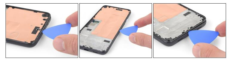
• Continue sliding the opening pick along the top, left, and bottom edges of your phone until all of the plastic tabs securing the back cover to the midframe are released.
