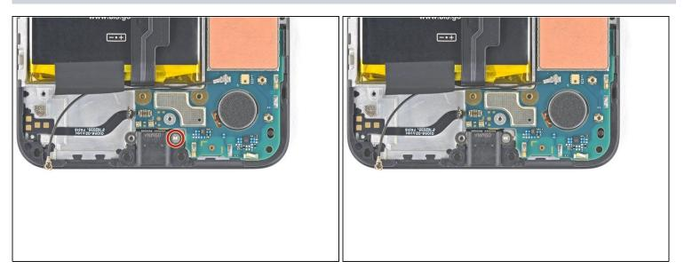
• Use a T3 Torx screwdriver to remove the 2.1 mm-long screw securing the charging port.
