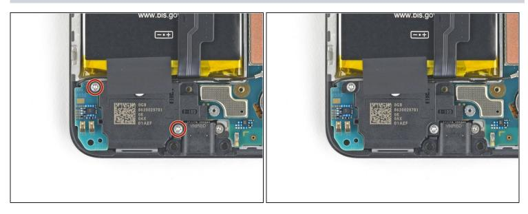
• Use a T3 Torx driver to remove the two 4.2 mm-long screws from the loudspeaker assembly.
