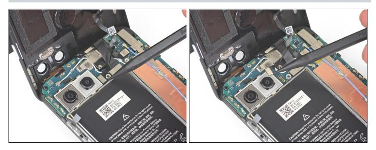
• Use the tip of a spudger to pry up and disconnect the fingerprint sensor cable.
