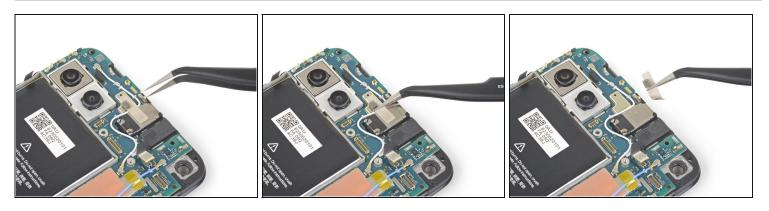
• Use a pair of tweezers to remove the tape on the earpiece speaker covering the antenna flex cable.
