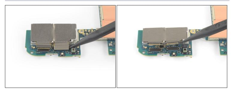
• Use the tip of a spidger to disconnect the right camera from the motherboard.
