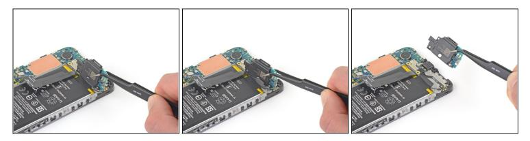
• Carefully peel the loudspeaker assembly up off the tape underneath it.
