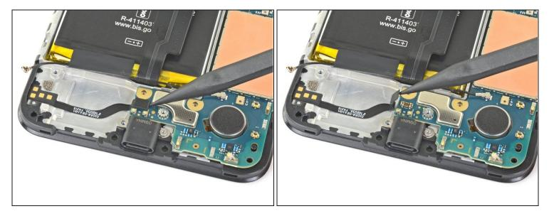
• Use the tip of a spudger to disconnect the loudspeaker cable from the motherboard.
