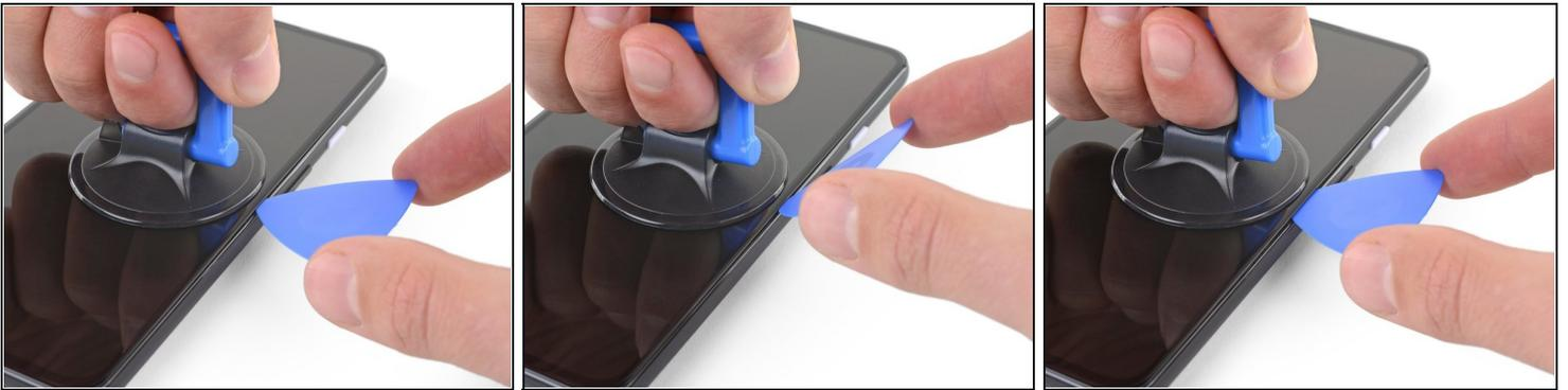
**i** This step shows how to insert your pick without damaging the OLED panel. Do this before slicing the adhesive.
