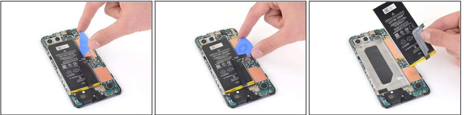
**⚠** Do not reuse the battery if it has been deformed or damaged, as doing so is a potential safety hazard. Replace it with a new battery.
