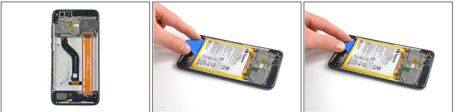
**⚠** The interconnect cable runs under the battery on the bottom right side. Make sure not to damage the cable during the following procedure.
