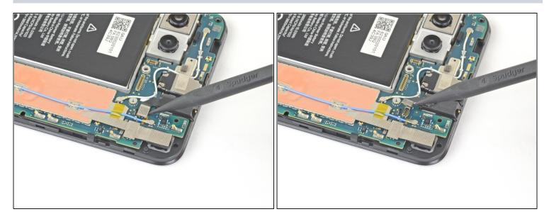
Use the tip of a spudger to disconnect the headphone jack from the motherboard.
