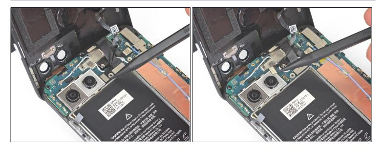
• Use the tip of a spudger to pry up and disconnect the fingerprint sensor cable.
