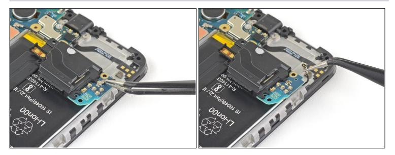
Use a pair of tweezers to disconnect the antenna cable from the loudspeaker assembly.
