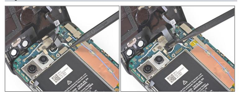
• Use the tip of a spudger to pry up and disconnect the front sensor array cable.
