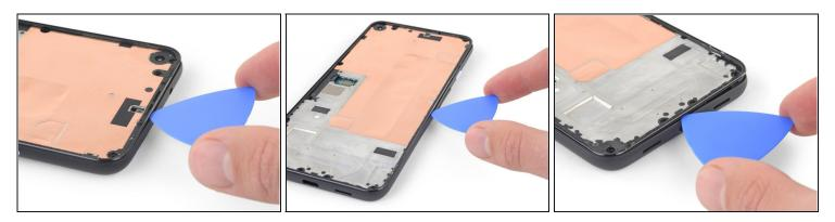
• Continue sliding the opening pick along the top, left, and bottom edges of your phone until all of the plastic tabs securing the back cover to the midframe are released.
