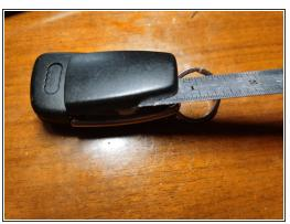
• Use a ruler or something less than or equal to 2 millimeters thick to poke through the slit at the bottom of the key fob and pry the key fob's shell open.
