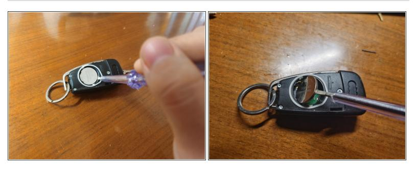
Poke a prying tool into the rectangular notch on the edge of the battery slot.
