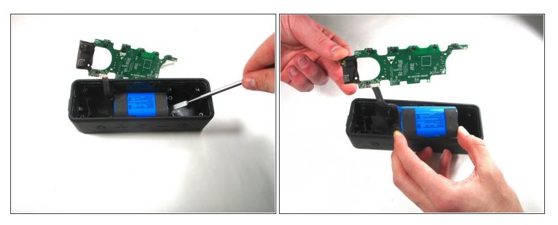
• Use a nylon spudger to remove the battery from the speaker casing.
