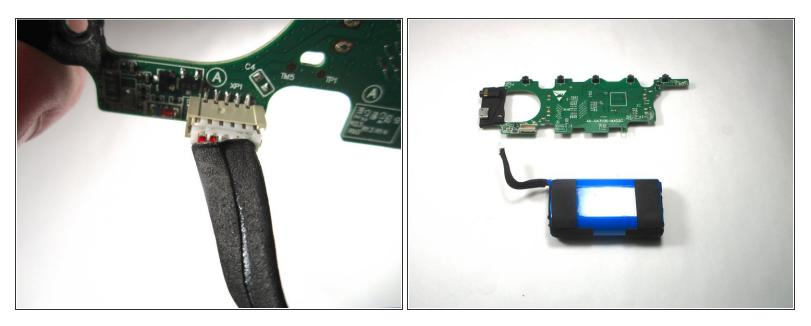
• Unplug the wire that connects the battery with the motherboard.
