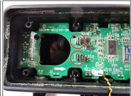
The speakers do not use wires so when replacing the speaker, make sure you align the metal prongs with the metal clips on the motherboard.
