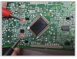
Turn the PCB to the other side. Find the soldering point of the battery as in the picture.
