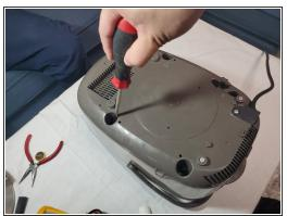
• Flip the device over and remove the four screws on the base using the Phillips #0 screwdriver.
