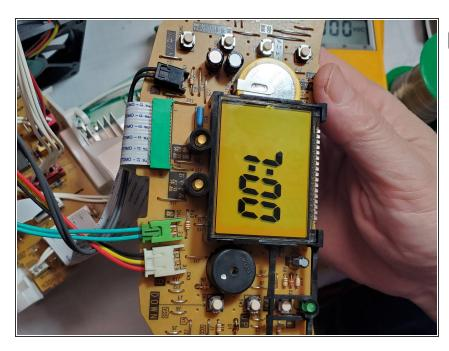
After soldering, you can check your result by making sure the front screen is displayed properly.
