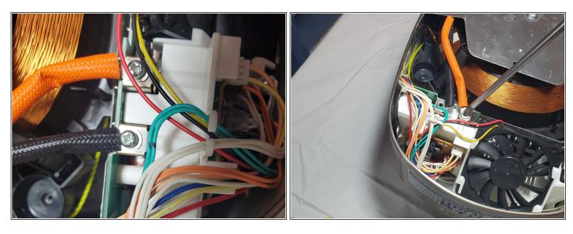
Remove the screws that connect the thick black and orange cables to the heat sink.
