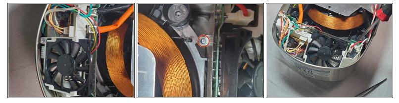
Remove the five screws connecting the heatsink to the device.
