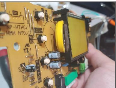
Desolder the two tabs then unplug the old battery.
