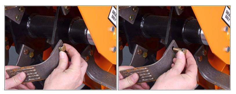
• Remove the two bolts holding the tine to the tine shaft.
