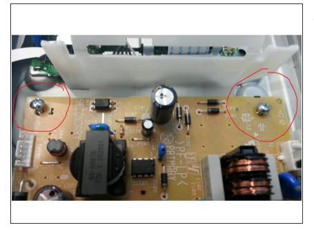
Unscrew two mounting screw for power supply. Slide forward and pull out for removal.
