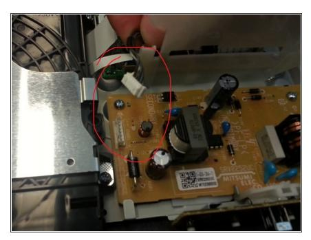
Release clip to remove 6 pin power cable.
