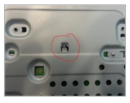
Release tab to remove plastic power supply shield.
