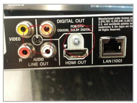
To completely remove the main board, locate screws on back of unit. Unscrew these 2 screws and then slide main board out.
