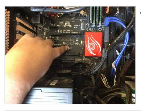
Insert battery back into position with the flat side facing upwards.
