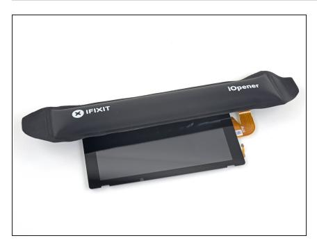
Heat the top edge of the screen assembly for around two minutes to help soften the adhesive holding the LCD panel to the digitizer.
