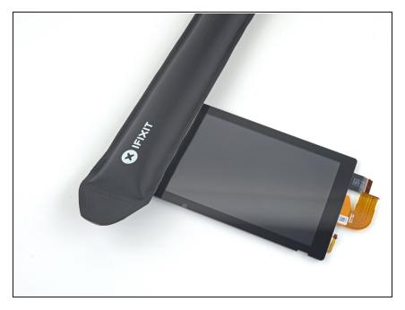
Heat the left edge of the screen assembly for around two minutes to help soften the adhesive.
