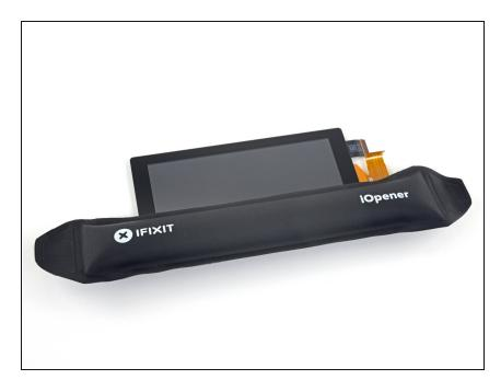
Heat the bottom edge of the screen assembly for around two minutes to help soften the adhesive.
