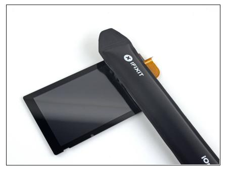
• Heat the right edge of the screen assembly for around two minutes to help soften the adhesive.
