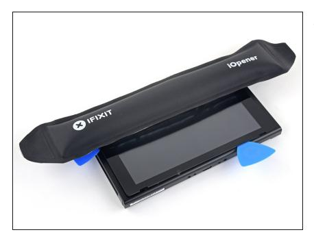
• Heat the top edge of the screen for around two minutes to help soften the adhesive.
