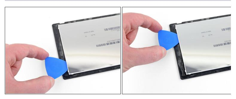
Insert and slide the opening pick along the left edge of the screen assembly to slice the adhesive.
