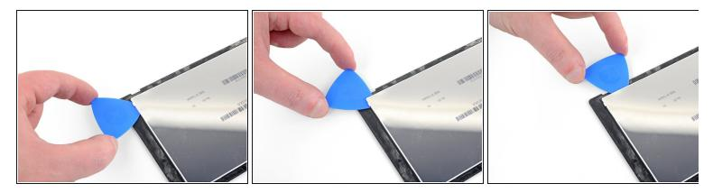
• Continue sliding the opening pick around the bottom-left corner of the screen assembly to slice the adhesive.
